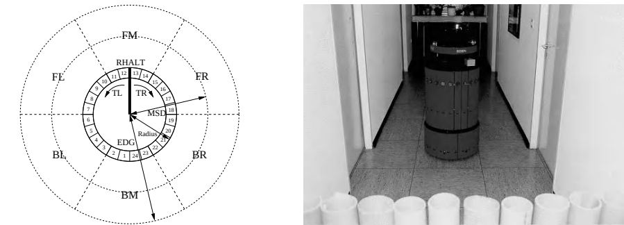
Fig. 1. Robot model seen from above with 24 sonar sensors combined to form six virtual sensors FL (front left), FM (front middle), FR (front right), BL (back left), BM (back middle) and BR (back right) which return the minimum distance of the corresponding 4 physical sonar sensors. The radius of the robot together with the minimum safe distance (MSD) and the desired edging distance (EDG) is also shown. The commands TL (turn left), RHALT (halt rotation) and TR (turn right) control the heading of the robot. The robot, a RWI B21, in its environment is shown on the right.
